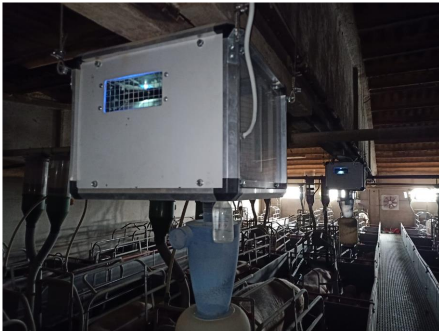
Figure 1. Prototype of the equipment with Cyclonic system. Airflow:100 m 3 /h.
